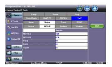
**VoIP Expert** – Generates industry standard wave files to verify MOS and R-factor values of upstream and downstream paths and includes QoS measurements such as packet jitter, packet loss, and delay. Compatible with all VeEX testers including VX1000 VoIP server software.
