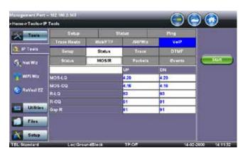
VoIP Call Expert – Emulates an IP phone and can place and receive calls using SIP or H.323 protocols. Comprehensive Codec support and call destination options verify voice encoding and translation provisioning. Real-time evaluation of subjective voice quality (MOS and R-factor) is made possible using the patented Telchemy® test method.
