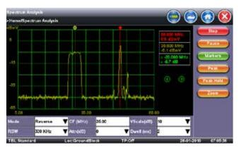
The CX350S is equipped with powerful spectrum analyzer features including a high dynamic range, markers, peak hold, variable resolution bandwidth (RBW) and variable dwell time (sweep speed) to help troubleshoot, identify and fix interference related problems.
