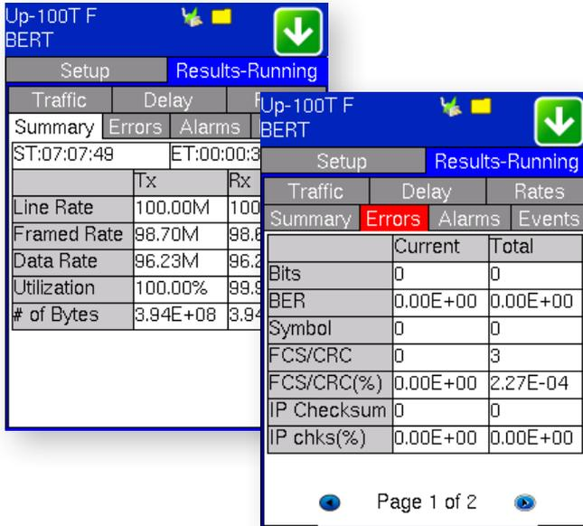
One traffic stream is transmitted across the network under test and bit-per-bit error checking is then performed on the received traffic. Service disruption measurements as well as CRC error checking are also performed. The BER test can be performed with a physical loop (or plug) at the far end (for a layer 1 circuit), or a second test unit or intelligent loopback device in Smart Loop or in Peer-to-Peer mode, for example, a low cost VeEX MLX100 loopback device.
