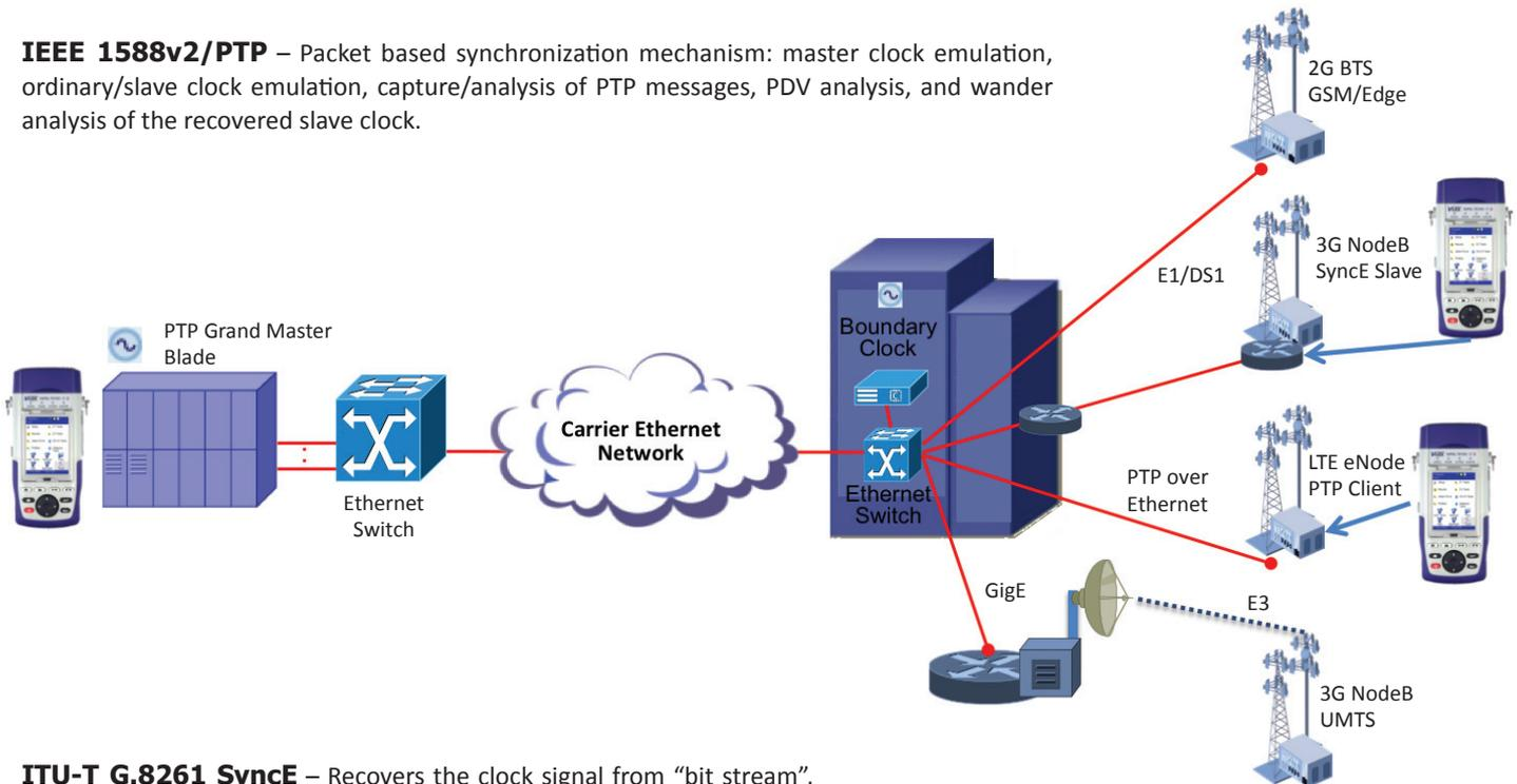
**ITU-T G.8261 SyncE** – Recovers the clock signal from “bit stream”, similar to traditional SONET/SDH/PDH. Wander and frequency measurement of the recovered slave clock.
