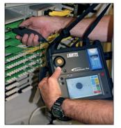
Analyzing connectors is as easy as capturing the images. Select analysis and touch the connector portion of the screen. **No calibration** is necessary. Just select Single mode or Multimode.
